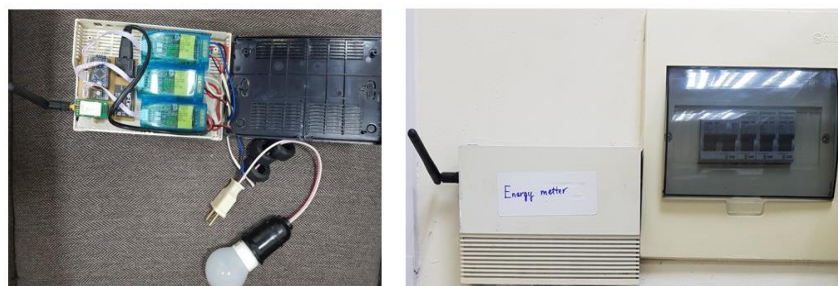
Figure 16. Energy meter in VHH (RF24 Mesh-Network).
